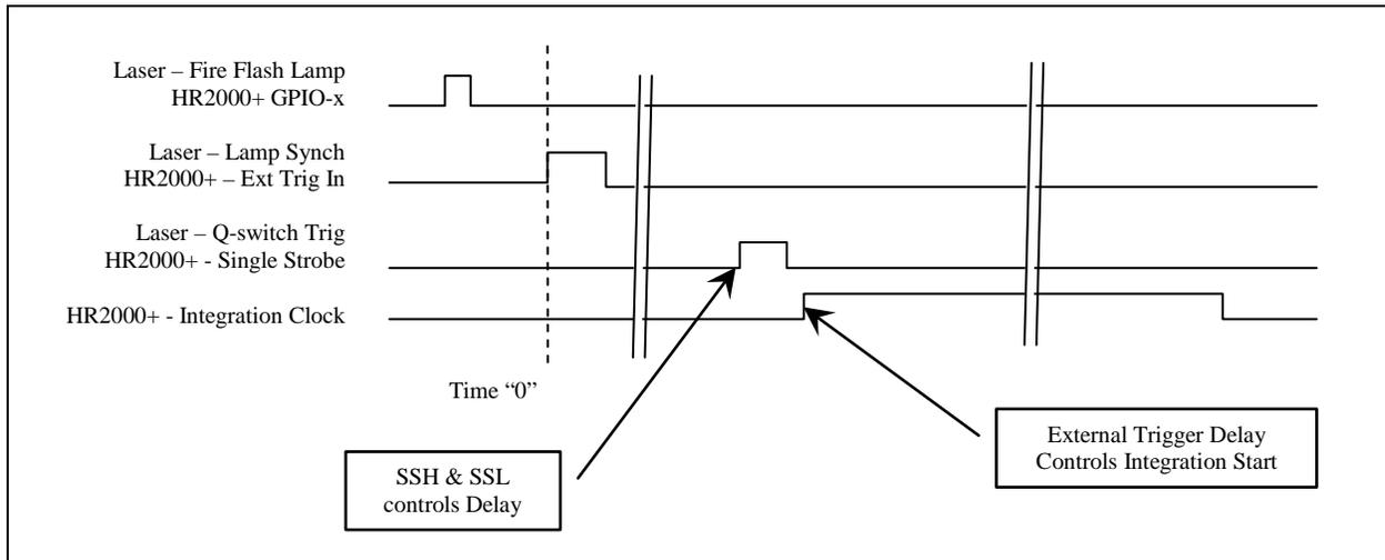
**Common Clock:** In order to reduce the jitter between the HR2000+'s, it is necessary to operate these on a common Clock. This is done by having the Master HR2000+ drive its Maser Clock Signal (default 2.4MHz – FPGA Register address 0), and having the other HR2000+'s use this Master Clock. This is done by configuring the master clock to drive the MCLK signal out the GPIO-1 pin (alternate function) and have the other spectrometers use this signal.
