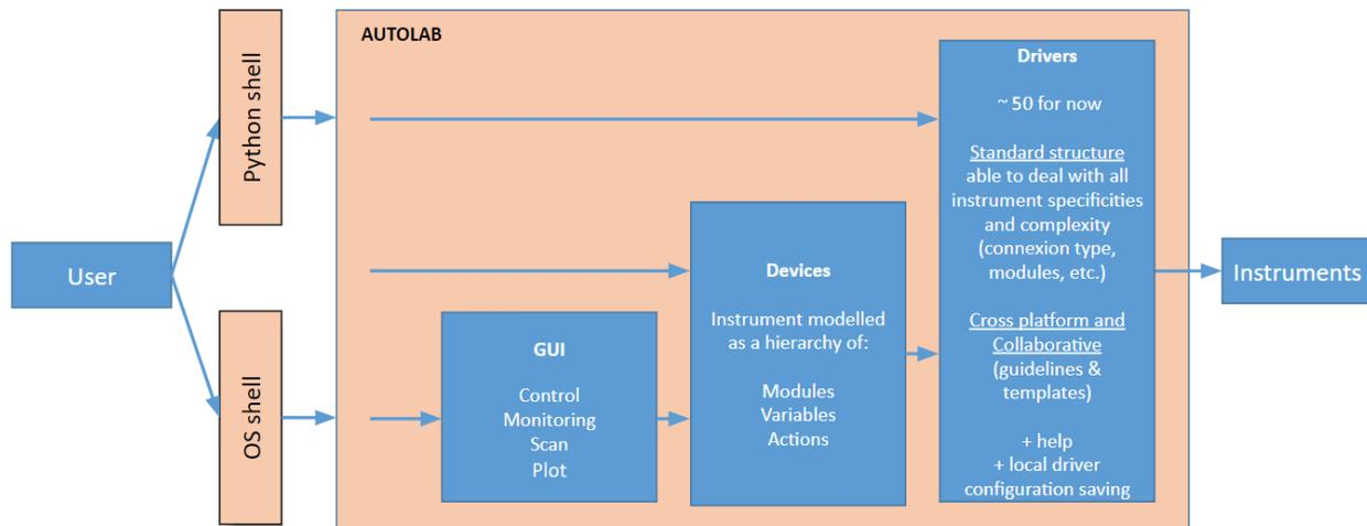
In this package, the interaction with a scientific instrument can be done through two different objects : the **Drivers**, or the **Devices**.
